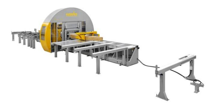
NC working centre with 6 continuous interpolating axis to process the 6 sides of the beams. Thanks to the innovative 360° rotating precision ring nut, the solid and glulam beams are automatically processed on 6 sides without the need to rotate them.
