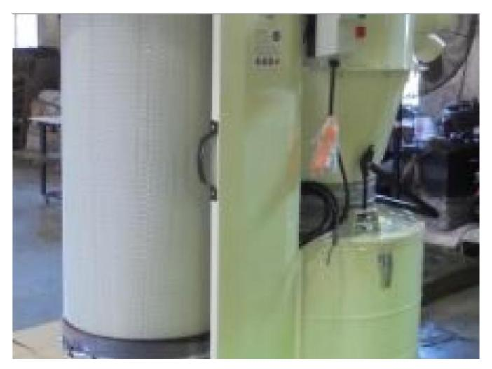
Two stage dust cyclone, This machine provides a combination of both power and portability with exceptional performance for both fine dust and particles.
