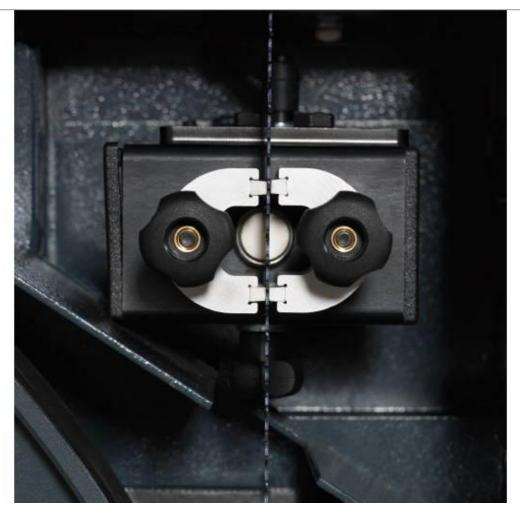
X-Life ceramic guides offer excellent cutting accuracy, blade stability and are extremely wear resistant. The four ceramic guiding blocks are able to be positioned directly adjacent to the blade with the flat surface ensuring reduced noise and less friction compared to traditional guides.
