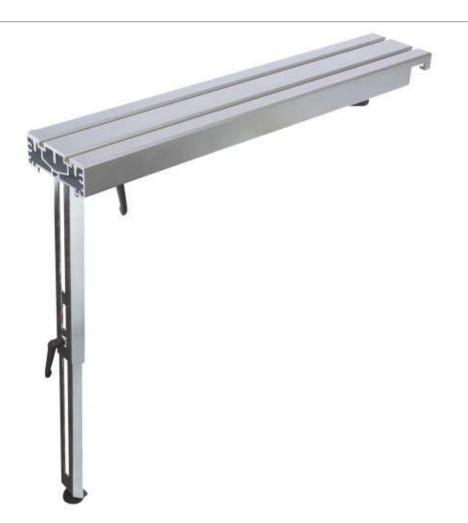
Aluminium table extension for use with Hammer machinery. Single-lever clamping system allows rapid installation for additional surface area as required. Includes support foot with height adjustment between 510 to 930mm. Suitable for all Hammer machine types with Hammer mounting rails.
