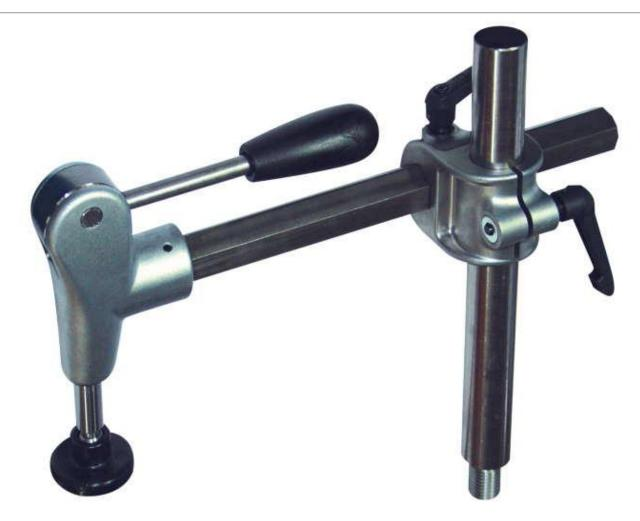
Cast-iron eccentric clamp which can be adapted for use on both Hammer and Felder sliding tables. Adjustable in both height and horizontal position it is suitable for neary all workpiece sizes and provides safe and comfortable work due to its high downforce pressure which prevents movement.
