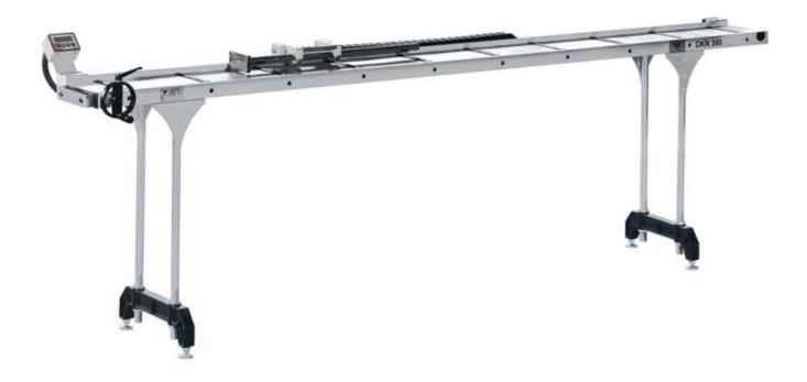
The DKN wind-along stop with digital readout.
