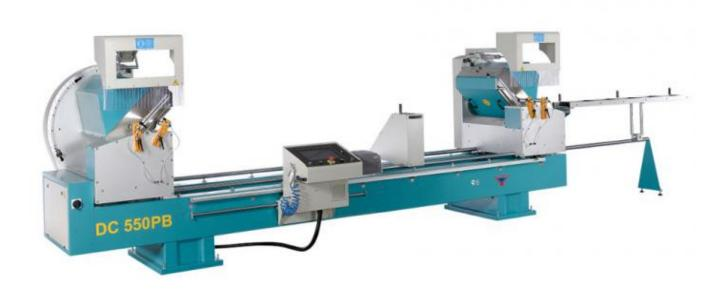
Yilmaz Double Mitre Saws offer the ultimate in cutting efficiency and versatility. They are able to cut large quantities of various profiles quickly and accurately without the costly mistakes commonly associated with "normal" single head cutting machines.
