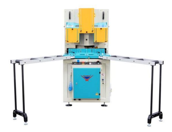
The VK 420 is designed for precise V cutting and  $90^{\circ}$  end notching with minimal off-cut sizes on aluminium, PVC and timber in one cut.
