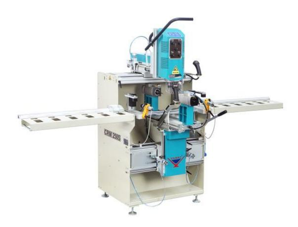
The CRM250S is a heavy duty copy router designed to machine on 3 sides of the profile without releasing the workpiece.
