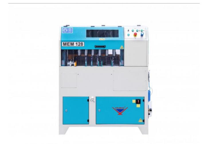
Yilmaz's MEM 128 is designed for end milling or notching multiple PVC and Aluminium profiles at the same time.
