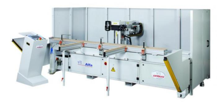
The Alfa is a highly flexible CNC milling machine for a quick and precise peparation of hung doors. It also offers the versatility of milling the preparation of stair stringers and louvre doors.
