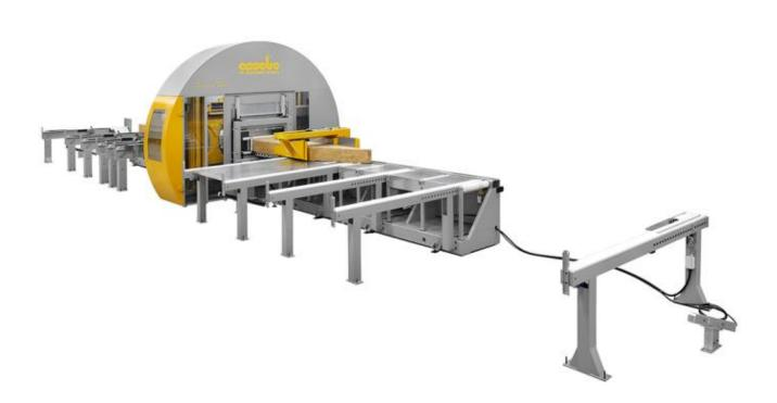
NC working centre with 6 continuous interpolating axis to process the 6 sides of the beams. Thanks to the innovative 360° rotating precision ring nut, the solid and glulam beams are automatically processed on 6 sides without the need to rotate them.
