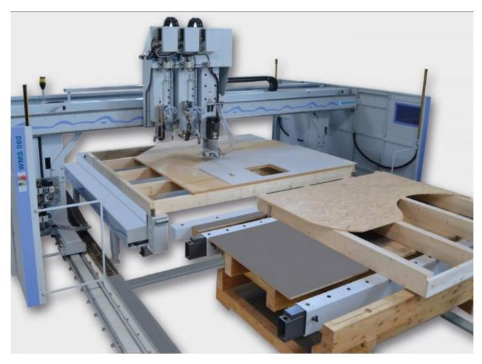
Weinmann's WMS 060 multifunction bridge allows you to create wall elements, roof elements, floor or gable elements at highest precision. The wide range of applications allows you to process a wide variety of wall structures and materials quickly and easily - all this at an excellent price-performance ratio!
