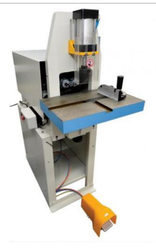
The HB301 is a compact horizontal single boring machine suitable for industrial or home workshop use. With a 1.5kW main motor and multiple drill gear heads, boring jobs are easier and safer, with extremely high accuracy.
