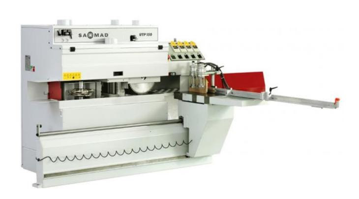
Through lateral movement of the saw blade and spindle, a quick change HSK 63 system and control panel layout, the UPT 150/1 provides maximum functionality, versatility and ease of use.
