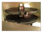
**Cope spindle tooling** Can be vertically or crosswise adjusted
