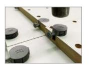
**Insert the Peanut 1** Use a mallet or hammer to insert the Peanut 1 flush
