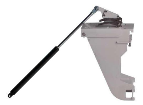
The powerfeeder tilt-away bracket clamps onto the F-channel mounts and allows a permanent fixutre of the powerfeeder. When the powerfeeder is not in use it is simply swung underneath the working table with gas strut assistance for lifting.
