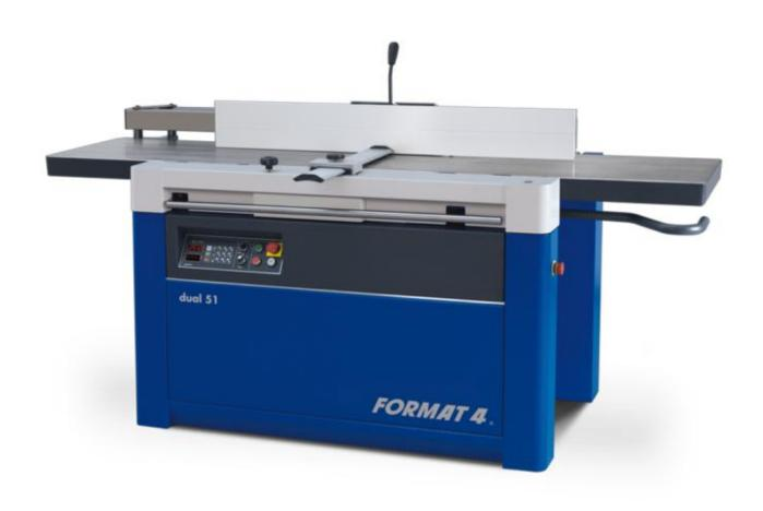
Are you looking for a planer-thicknesser that meets your professional requirements in regards to precision, reliability and ease of use? The Format4 dual 51 sets new standards in all areas. Solid ribbed planing table and a 4 column thicknessing table guide system ensure high stability.
