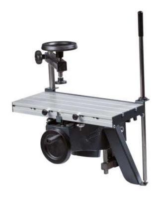
Attachment for Hammer A3 and C3 series machines for additional function of mortising and drilling via the planer cutterblock. Height adjustable table with handwheel and movement controlled by hand lever. Includes workpiece clamp.
