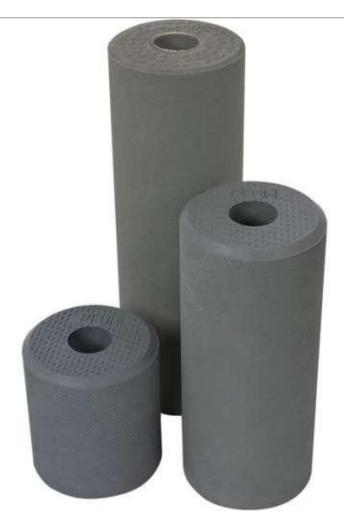
Grey foam rubber roller with a ribbed and non-porous surface suitable for white glues, and glues with added hardener (kaurit glue). This roller gives a thinner glue application than other rollers such as for veneer work with coarse-pored veneers.
