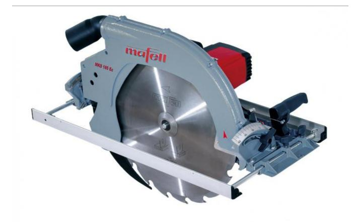
The Mafell MKS 185Ec carpenter's portable circular saw uses ultra-modern die-cast magnesium alloys to achieve an extraordinary weight/performance ratio. Weighing only 16.1kg, the MKS 185Ec accurately and powerfully makes 185mm cuts like no other saws in its class.
