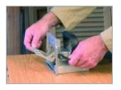
Angle and height-adjustable front fence with graded scale
