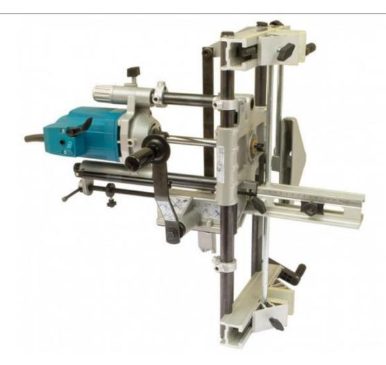
The FC116U is specially designed for quick, precise morticing on doors or other elements, either at the worksite or in the workshop.
