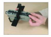
Micrometric measure for easy adjustment of strip width
