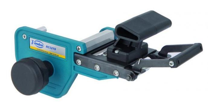
The RC321S Hand End Trimmer is designed for cutting excess PVC, melamine, polyester, veneer etc. It trims tapes up to 45mm wide and 3mm thick, at both ends of the panel. This trimmer provides a clean and exact cut, avoiding damage to the panel already banded.
