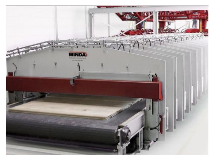
The TimberPress X300 is designed for producing CLT (Cross-Laminated Timber) in dimensions of up to 18.0m length and 3.5m width, with custom dimensions available on request. These hydraulic CLT presses are appropriate for high production factories.
