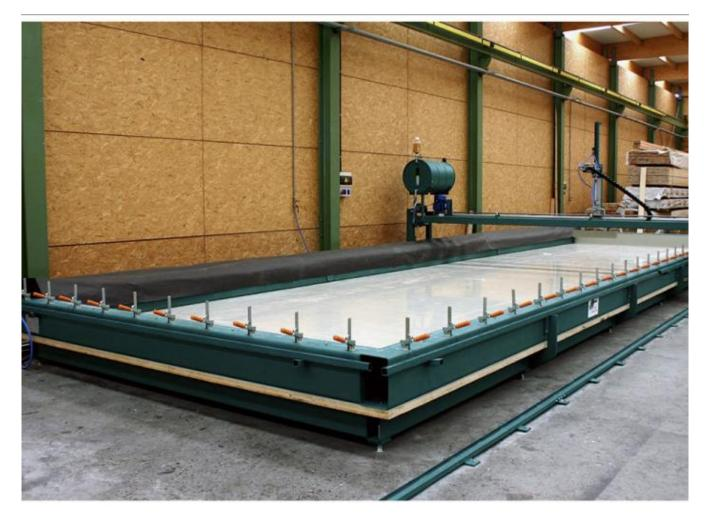
The most affordable entry to Cross Laminated Timber (CLT) production, Swiss-made Woodtec vacuum presses are proven worldwide. For more than 10 years companies around the globe have been producing large panels with the Woodtec vacuum press technology, with around 40 machines installed. The advantages are attractive:
