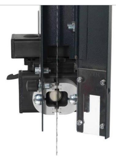
X-Life ceramic guides offer excellent cutting accuracy, blade stability and are extremely wear resistant. The four ceramic guiding blocks are able to be positioned directly adjacent to the blade with the flat surface ensuring reduced noise and less friction compared to traditional guides.
