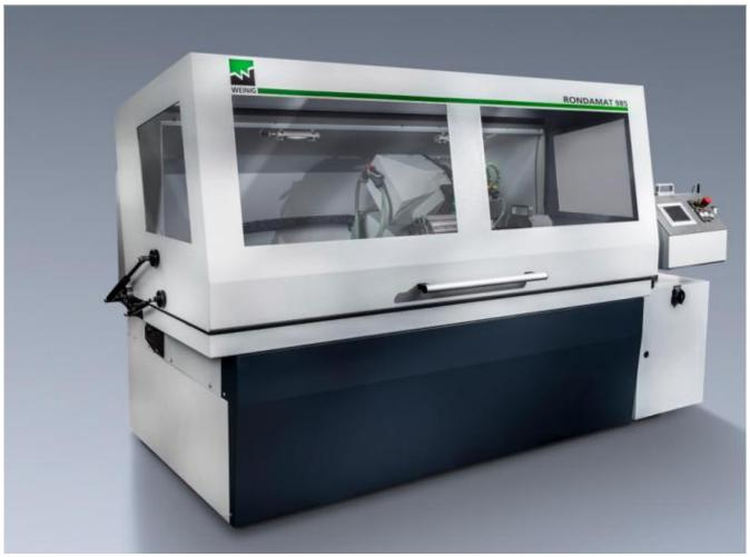
The Rondamat 985 is the ultimate solution for precision sharpening of planing cutterheads, accommodating widths of up to 720 mm. Whether you're working with a conventional cutterhead, hydro cutterhead, or a shaft cutterhead, this versatile machine has you covered. What sets it apart is its unique capability to sharpen knives directly within the cutterhead, making it possible to subsequently align hydro clamped tools with ease.
