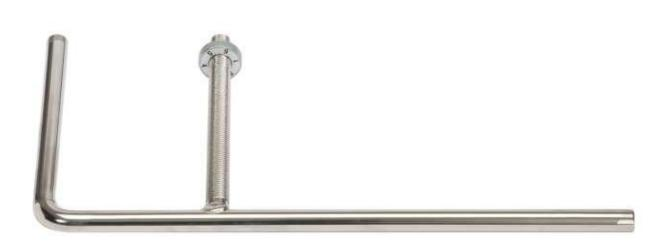
The Universal Support is the basis for all Tormek jigs. The square cut Acme style thread prevents damage by the locking screws and a Micro Adjust with scale gives precise setting of the edge angle and cutting depth to replicate exact angles every time.
