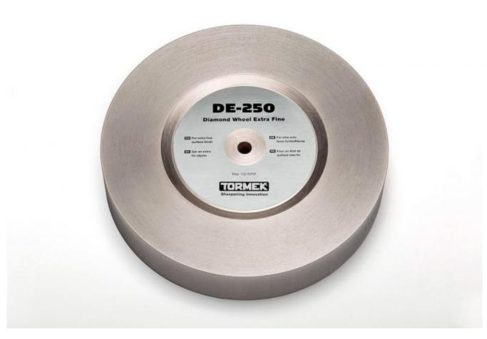
The Tormek Diamond Wheel Extra Fine with a grit size of 1200 leaves an extra fine finish and is especially suitable for carving tools and knives when the need for steel removal is minimal.
