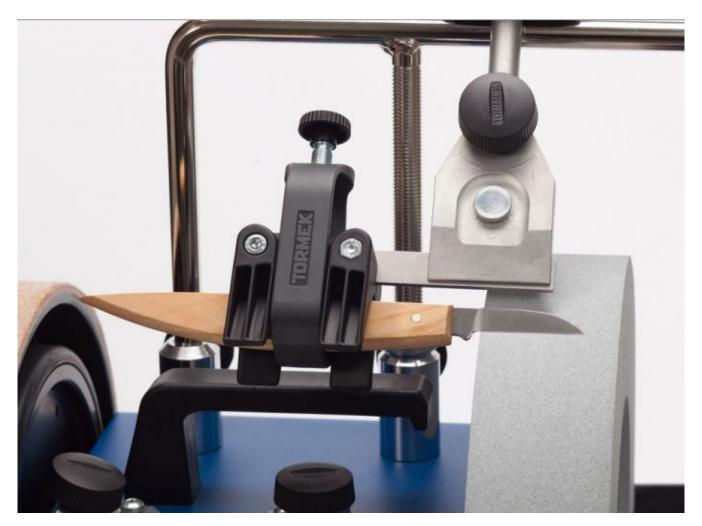
The Small Knife Jig SVM00 from Tormek can handle those really small knife blades which, up until now, have been difficult to sharpen. Normally they have been sharpened freehand but every time it has been a challenge to get a consistent shape and almost impossible to control the edge angle.
