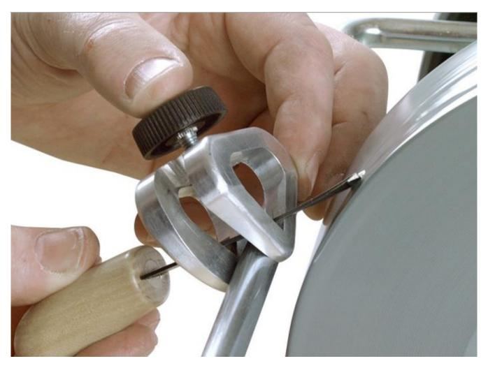
The SVS38 is for straight-shanked tools, such as wood chisels, carving gouges and tools for power carvers. Flanges ensure a 90° positioning of the tools towards the grindstone. Copes with tools down to 45mm ( $1\frac{3}{4}$ ") length and max width 38mm ( $1\frac{1}{4}$ ").
