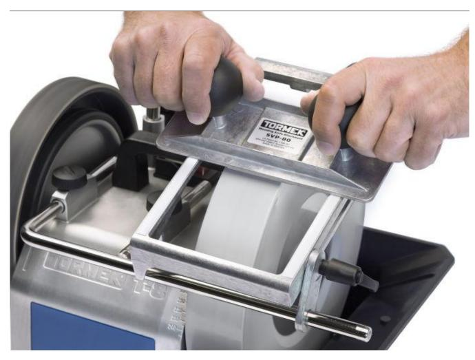
The SVP80 Moulding Knife Attachment is for all shapes and makes of moulding knives with 24, 30 or 38mm distance between guide holes. It sharpens the face of the blade and can therefore work on any shape.
