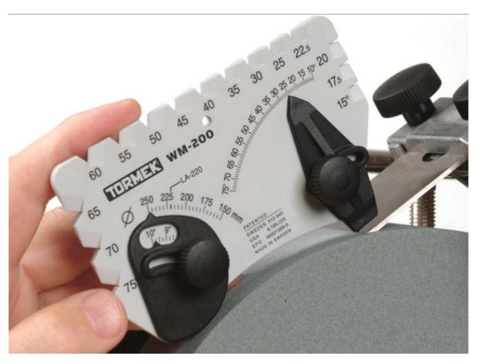
The AngleMaster sets and measures the edge angle. It is adjustable to any stone diameter from  $\emptyset$  250mm or 10" down to  $\emptyset$  150mm or 6", and measures from 10° to 75°.
