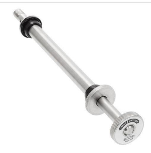
The shaft, washer and EzyLock nut are all made of stainless steel to resist rust. The EzyLock system ensures that the grindstone is held securely with no danger of unwinding while also requiring no tools to mount or loosen the grindstone. A special pitch on the left hand thread causes the rotation of the wheel to tighten the nut to the correct torque.
