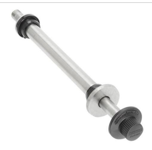
The shaft is made of stainless steel and the EzyLock nut of composite material to resist rust. The EzyLock system ensures that the grindstone is held securely with no danger of unwinding while also requiring no tools to mount or loosen the grindstone. A special pitch on the left hand thread causes the rotation of the wheel to tighten the nut to the correct torque.
