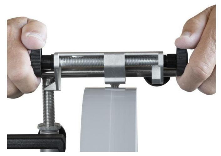
With the Tormek TT50, you can true and dress your grindstone exactly round and flat. It mounts and locks instantly on the Tormek Universal Support. The tool is guided by the Universal Support, which also guides the jigs. This ensures that the stone surface is always parallel to the tool fitted in the jig.
