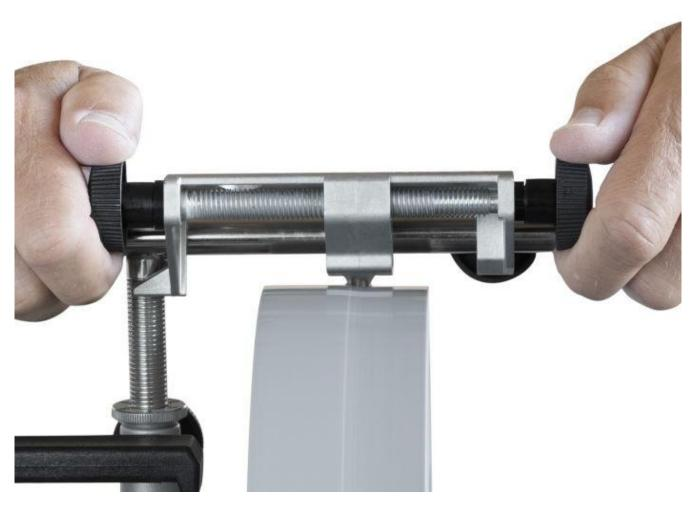
With the Tormek TT50, you can true and dress your grindstone exactly round and flat. It mounts and locks instantly on the Tormek Universal Support. The tool is guided by the Universal Support, which also guides the jigs. This ensures that the stone surface is always parallel to the tool fitted in the jig.
