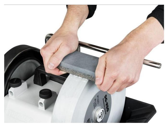
The SP650 Stone Grader is used for changing the function of the grindstone. The fine side grades the stone for a 1000 grit finish. The coarse side of the grader reverses the stone to normal 220 grit for faster grinding. The SP650 also activates a glazed grinding stone.
