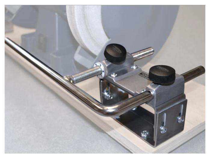
No matter which grinding machine you use, the most difficult part in sharpening woodturning tools is to exactly replicate the shape and the edge angle. The Mounting Set BGM100 makes the patented Tormek woodturning system jigs available for those who want to use their existing bench grinder.
