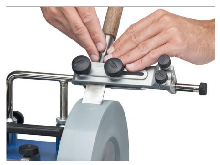
With the SE77 Square Edge Jig, it is easy to set your wood chisels and plane irons for sharpening to a square corner. The design gives you the best conditions for a successful sharpening with the highest precision over the final result. You can also set the jig for a slightly convex shape.
