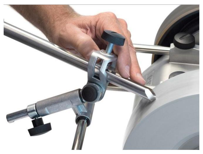
The SVD186 Gouge Jig is used for an exact replication of the shape on fingernail-shaped turning gouges. You can also grind straight and curved V-tools.
