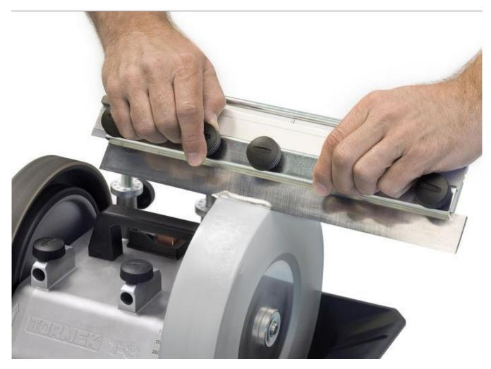
The SVH320 is for sharpening blades of any length. Blades longer than 270mm ( $10\frac{1}{2}$ ") are relocated in the blade holder and ground in two steps. The grinding depth can be set within 0.1 mm (0.004").
