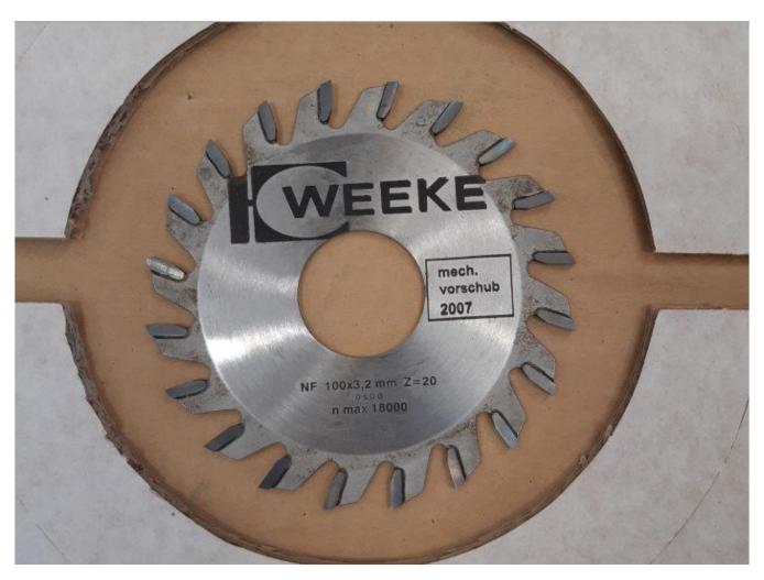
Sawblade for grooving with maximum rotational speed 18,000rpm.
