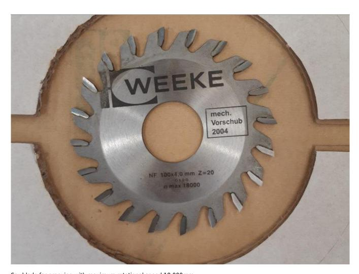
Sawblade for grooving with maximum rotational speed 18,000rpm.
