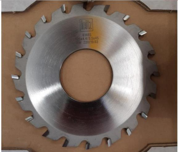
Conical scoring blade by Leitz originally brought in for use with HOMAG & Giben beamsaws.
