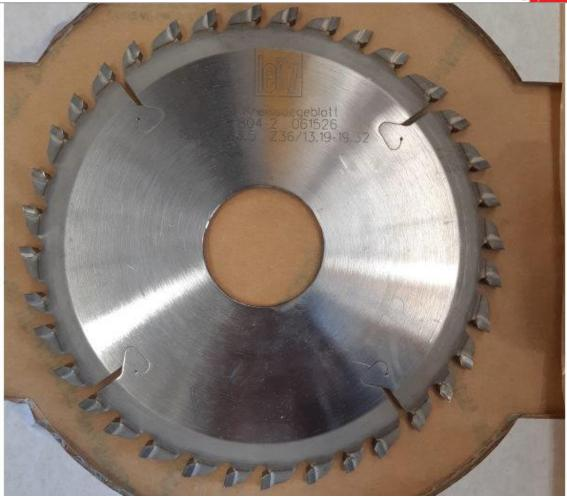
Conical scoring blade by Leitz. Originally brought in for use with Holzma beamsaws.
