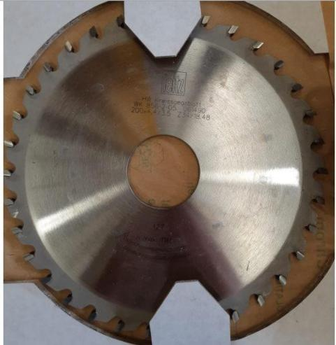
Conical scoring blade by Leitz originally brought in for Holzma beamsaws.
