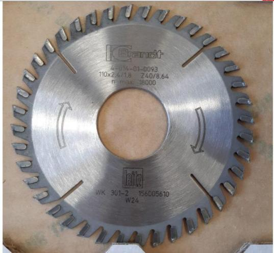
Cutoff blade by Leitz, originally designed for end trimming saws on Brandt Edgebanders.
